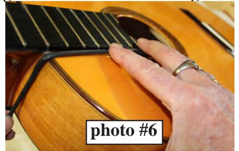
**Photo # 6** - The gooseneck is positioned alongside the soundhole, and bent down the side (rib) of the guitar. There should be a sharp bend where the top meets the side
